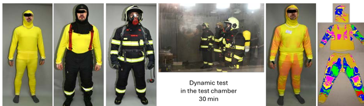
Figure 2 (a-f) Testing of structural integrity of firefighter protective suit in toxicologic chamber
