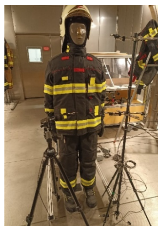
Figure 2. Measurement of I_T and R_{eT} using 34-zones thermal manikin Newton at BUT, Czech Republic
