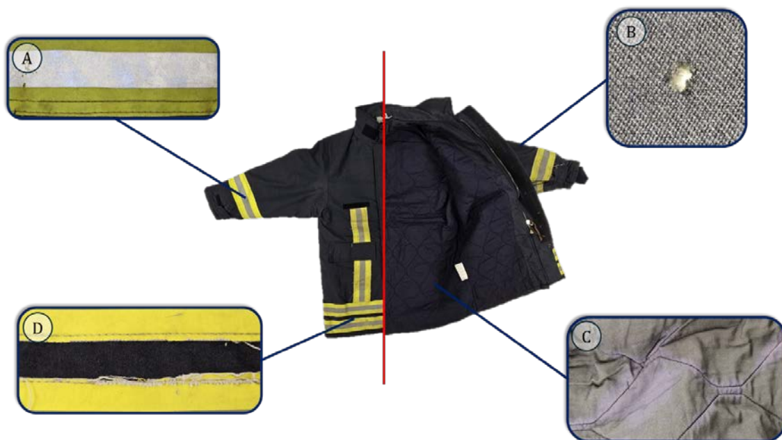
Figure 1. Used firefighter jacket with various signs of use: A -blind reflectors, B -extinguishers, C -washed out inner lining with sweat stains, D -broken seams and frayed edges
