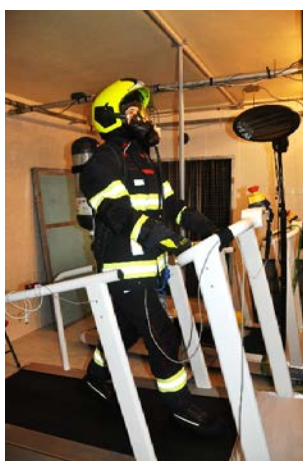
Figure 1. Proband in in climatic chamber at 35 °C, walking on treadmill
