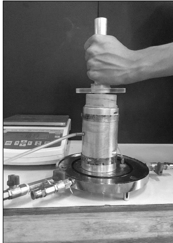
b. Compaction of layers
