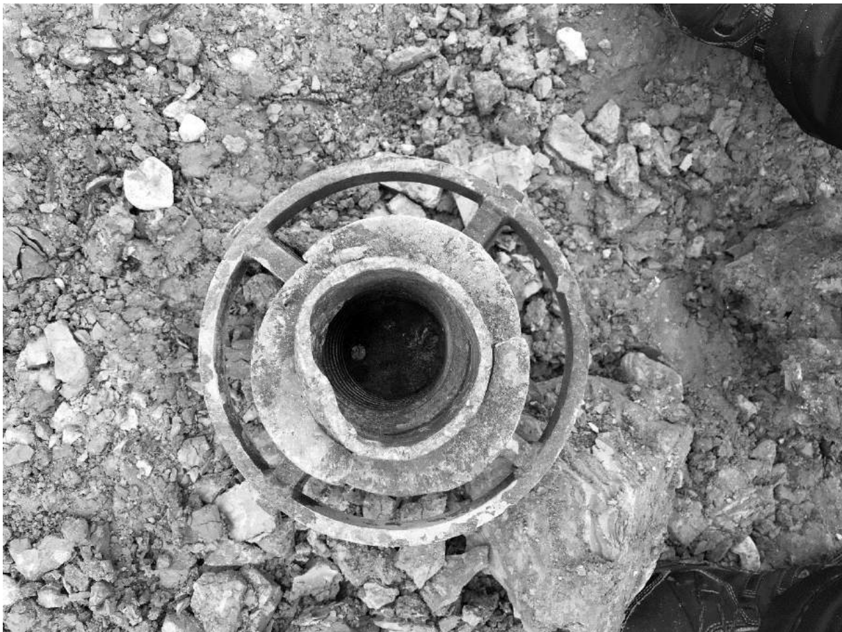
Figure 2. Shear of the anchor steel bar
