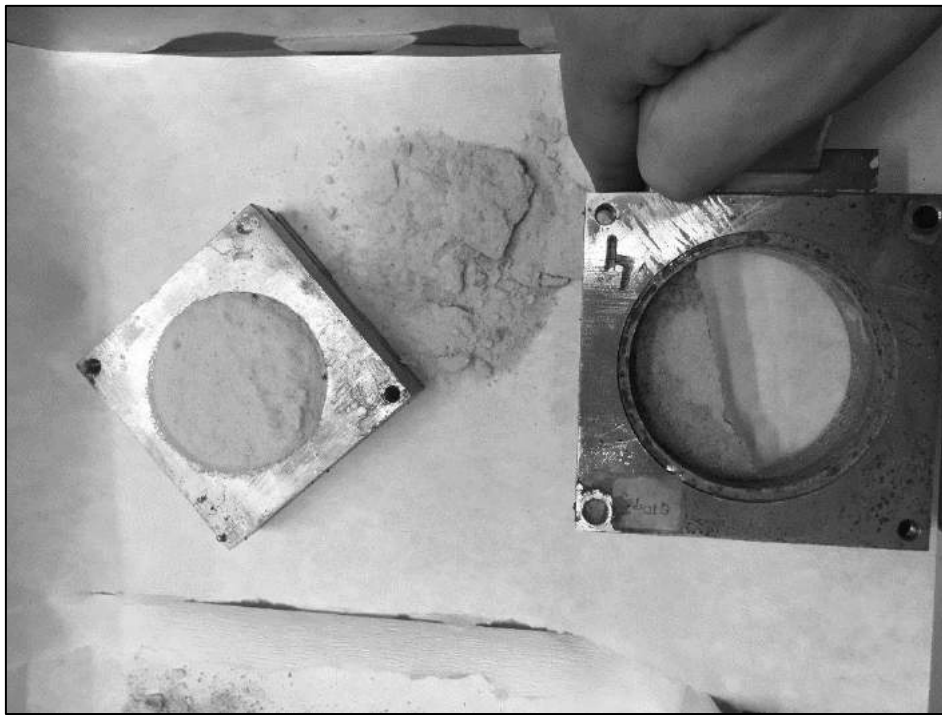
Figure 1. Crust layer observed after drying process
